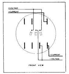
D5S-7, D4S-7, E1S-7E 3-phase, 4-wire, delta self-contained — Right Stator Test. FORM 15S
