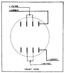
D5S-2, D4S-2, E1S-2E 1-, 2-, or 3-phase, 3-wire, self-contained and transformer-type — Right Stator Test. FORM 5S
