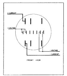
D5S-8, D4S-8, E1S-8E 3-phase, 4-wire, wye transformer type — Left Stator Test. FORM 6S
