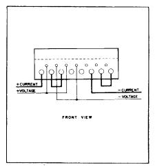
D5A-7, D4A-7, E1A-7E 3-phase, 4-wire, delta transformer-type -- Combined Stator Test. FORM 8A
