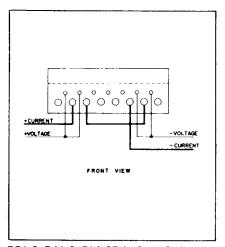
D5A-2, D4A-2, E1A-2E 1-, 2-, or 3-phase 3-wire, transformer-type — Combined Stator Test. FORM 5A
