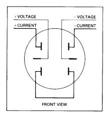
D5S, 3-wire, 6-terminal transformerrated—two CTs test. Form 4S
