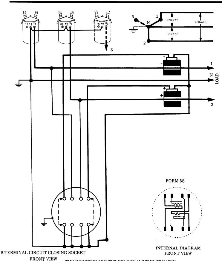
THE REGISTER MULTIPLIER EQUALS THE CT RATIO FOR SECONDARY-RATED METERS
