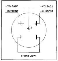
D5S, 3-wire self-contained—meter test. Form 2S
