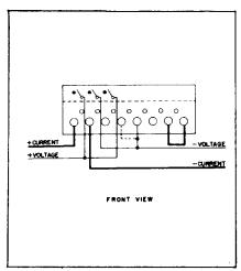
D5A-7, D4A-7 3-phase, 4-wire, delta self-contained — Left Stator Test. FORM 15A
