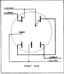
D5S-5, D4S-5, E1S-5E 1-, 2-, or 3-phase, 3-wire, self-contained — Combined Stator Test. FORM 12S
