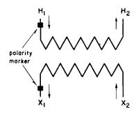
Figure 4 - Arrows indicate instantaneous relative direction of currents in the windings.
