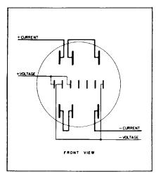
D5S-7, D4S-7, E1S-7E 3-phase, 4-wire, delta transformer-type — Combined Stator Test. FORM 8S
