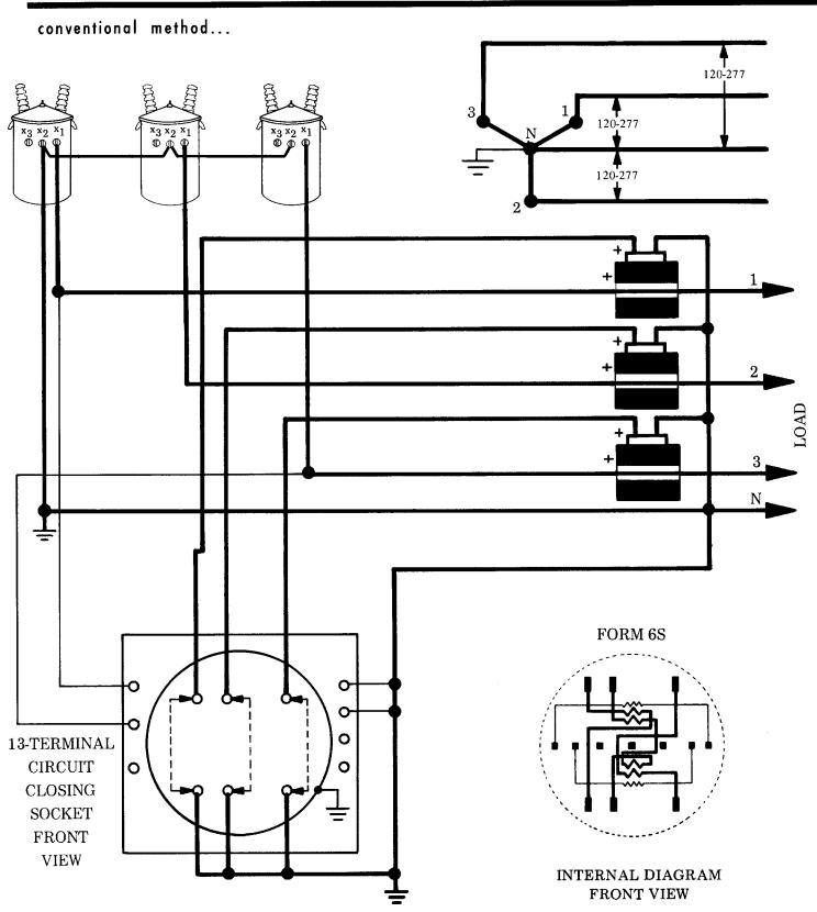
THE REGISTER MULTIPLIER EQUALS THE CT RATIO FOR SECONDARY-RATED METERS
