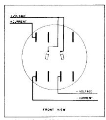
D5S-8, D4S-8, E1S-8E 3-phase, 4-wire, wye self-contained — Left Stator Test. FORM 14S
