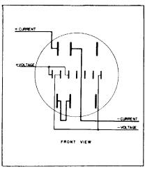
D5S-7, D4S-7, E1S-7E 3-phase, 4-wire, delta transformer-type — Left Stator Test. FORM 8S
