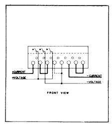
D5A-7, D4A-7 3-phase, 4-wire, delta self-contained — Combined Stator Test. FORM 15A
