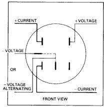
D5S, 2-wire, 5-terminal transformerrated—CT test. Form 3S
