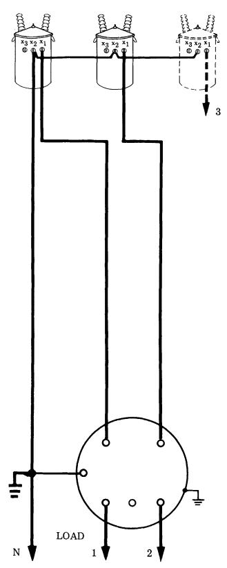
5-TERMINAL NON-CIRCUIT CLOSING SOCKET FRONT VIEW
