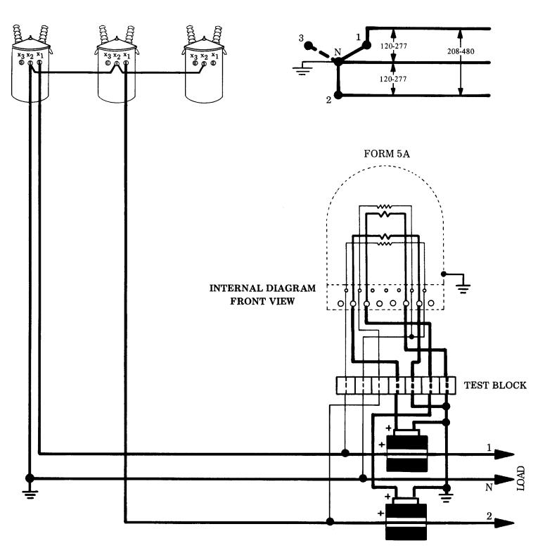
THE REGISTER MULTIPLIER EQUALS THE CT RATIO FOR SECONDARY-RATED METERS
