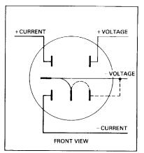
D5S, 2-wire, 4- or 5-terminal transformer-rated—CT and VT test. Form 3S
