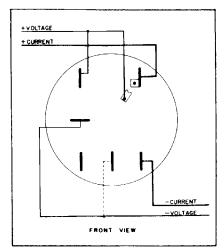
D5S-5, D4S-5, E1S-5E 1-, 2-, or 3-phase 3-wire, self-contained — Right Stator Test. FORM 12S
