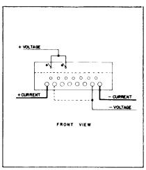
D5A-2, D4A-2 1-, 2-, or 3-phase, 3-wire, self-contained — Left Stator Test. FORM 13A
