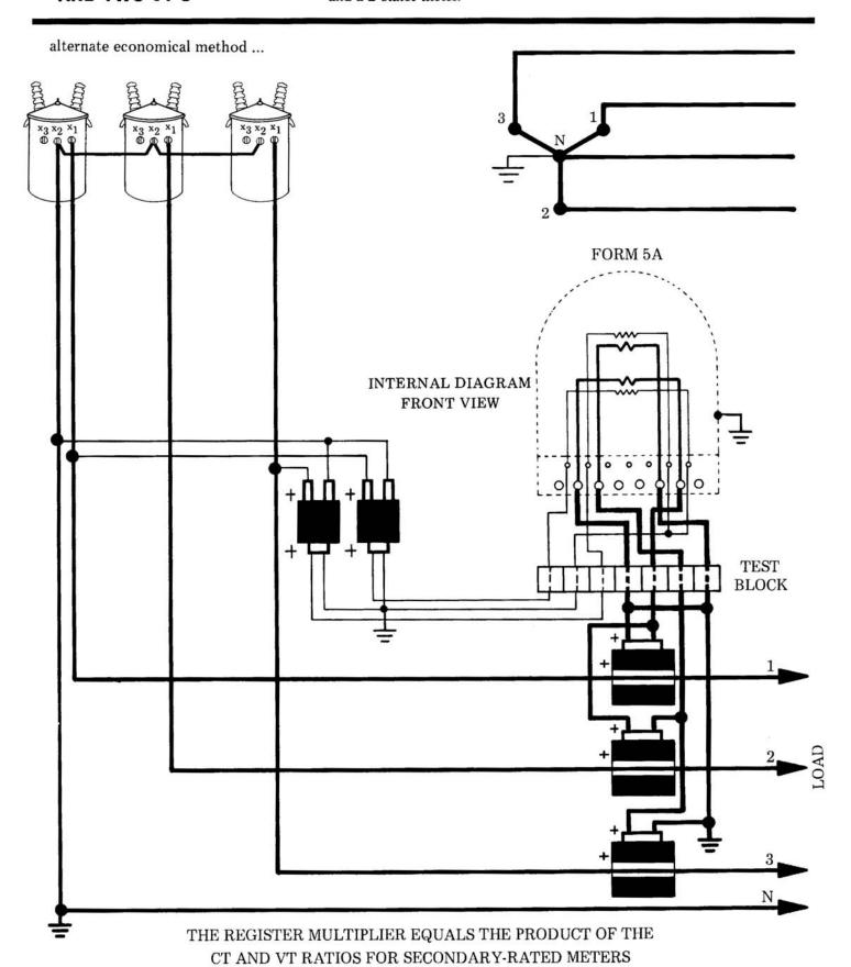
Measurement of energy on a three-phase, four-wire Wye service with 3 CT's, 2 VT's, and a 2-1/2-stator meter.
