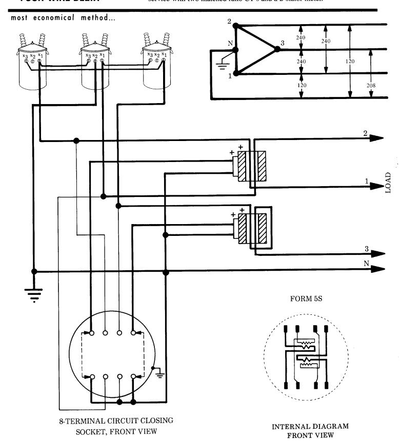
THE REGISTER MULTIPLIER EQUALS 1/2 CT RATIO FOR SECONDARY-RATED METERS
