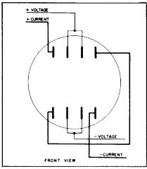
D5S-2, D4S-2, E1S-2E 1-, 2-, or 3-phase, 3-wire, self-contained and transformer-type — Combined Stator Test. FORM 5S
