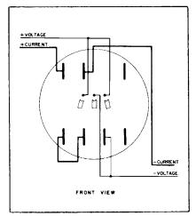
D5S-7, D4S-7, E1S-7E 3-phase, 4-wire, delta self-contained — Left Stator Test. FORM 15S
