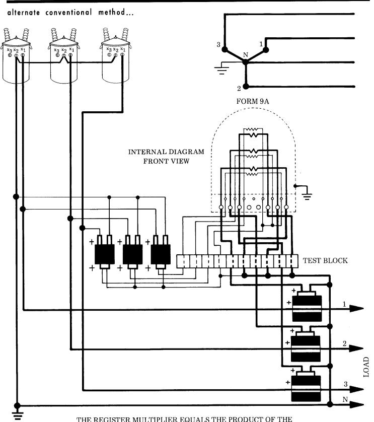
THE REGISTER MULTIPLIER EQUALS THE PRODUCT OF THE CT AND VT RATIOS FOR SECONDARY-RATED METERS
